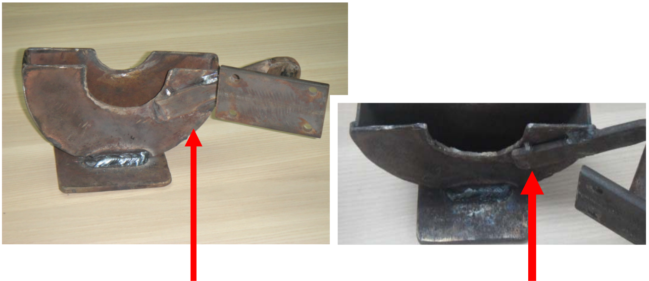
Gambar 8 : Plat besi bersaiz 5mm x 110mm x 25mm dipotong
